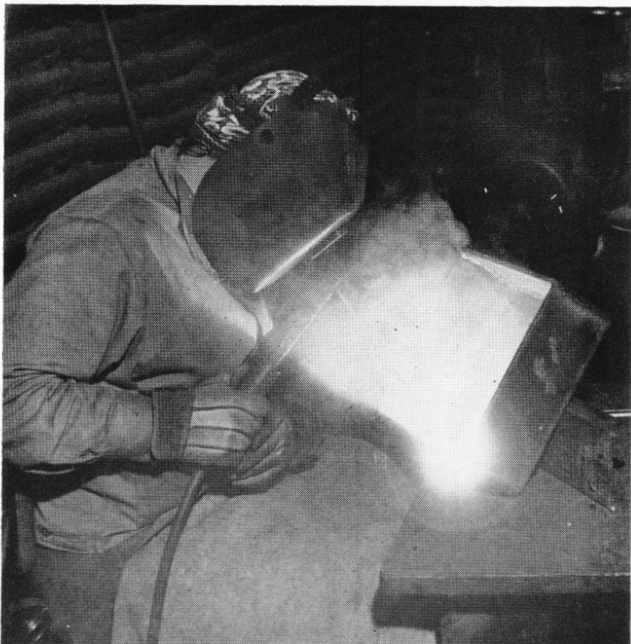
Sue M. Colangelo is electric welding with one of the A-C Current machines recently purchased for the new Welding Shop. The A-C machines are popular with the operators. Some state that they can do quicker work and perform better corner jobs with them.
