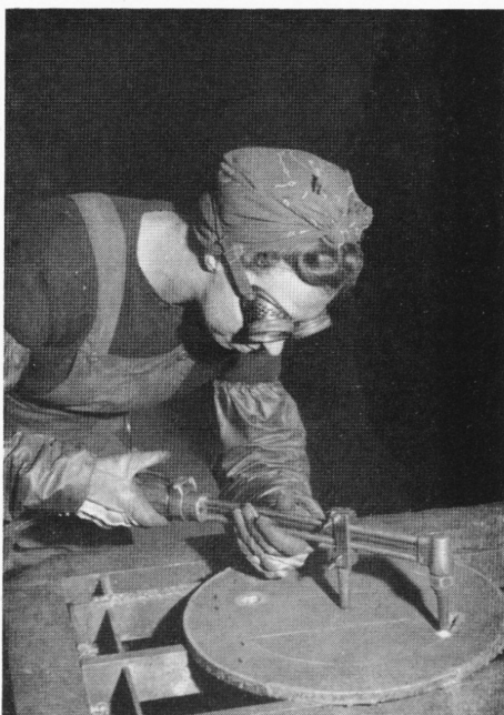
Using a burning torch, Eve Brunelli is cutting a circle in a steel plate. This job takes a good deal of skill. The Welding Shop can cut plate steel up to a six-inch thickness.
