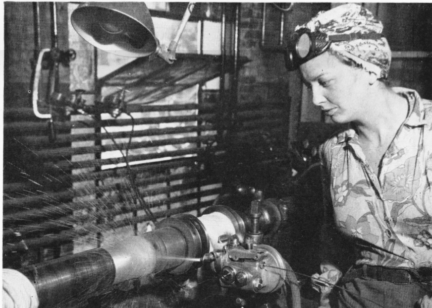
Jo Ann Foley is metalizing — another new process adopted by the Welding Department. Wire of applied metal is melted within the torch and sprayed upon the work much as paint is sprayed. Metalizing is used to rebuild worn, or to add metal to other, surfaces. Original or almost any desired metal can be applied by this method.
